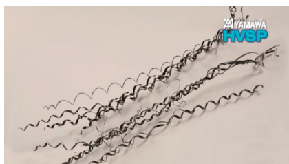
Ejected chips by large size taps
