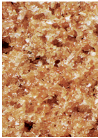
Open or closed: less dense wheels take a lot of coolant and cut large volumes away quickly. Dense structures last for a long time, for applications such as profile grinding. Whatever the case, we will find the optimum solution for your application
