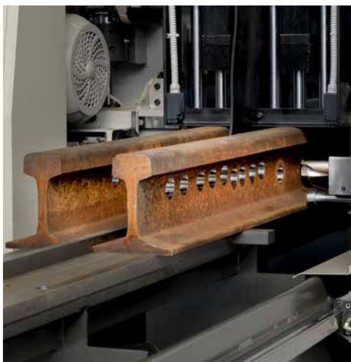
Impianto speciale per taglio e foratura binari con diametro massimo 40 mm Special system for cutting and drilling tracks with a maximum diameter of 40 mm
