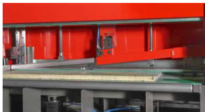
Pattino guidalama mobile – Movable blade guide
