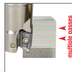
no signs on shouldering wall
